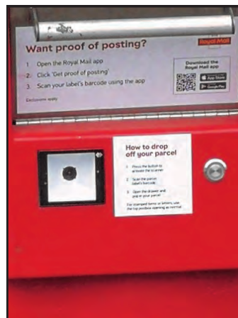
The front panel of the New Style Postbox as at the left. The handle at the top opens the larger parcel aperture.
